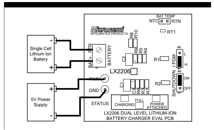
Figure 3 - LX2206 Typical Test Hookup
